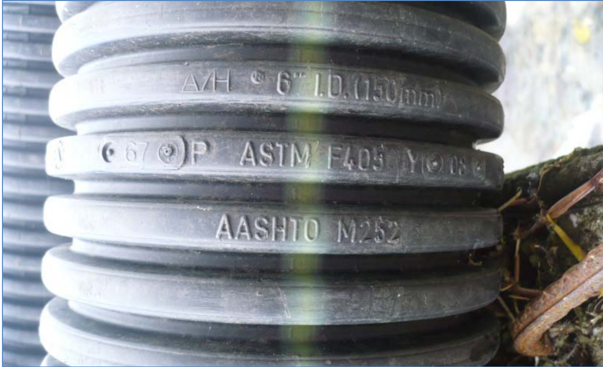
Figure 3.6: Black Corrugated Pipe (Walker 2011)
