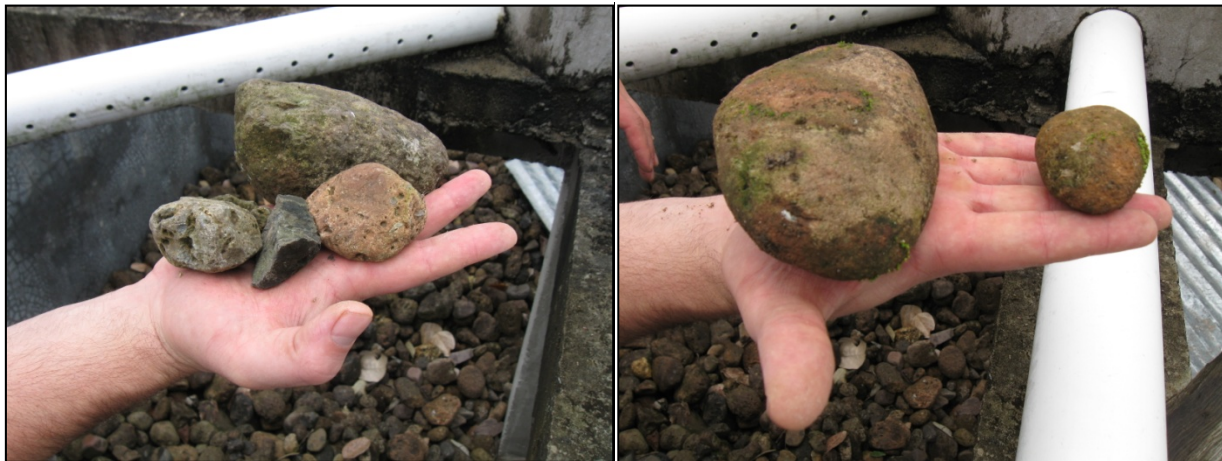
Figure 3.14: Las Casetas Trickling Filter Media (Puckett, 2011)
